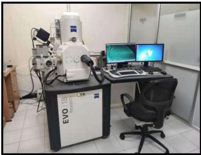
**Carl ZEISS EVO 18- Germany-** Operating modes Secondary electron (SE) and Backscattered electron (BSD) Modes. Up to 200 nm resolution depends up on samples. It is attached with AMETEK Team V.4.3 EDS detector.
