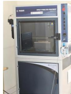
Ultrasonic Spray Pyrolysis unit
